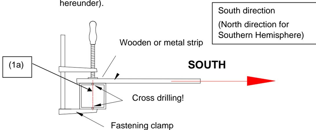
During drying-procedure of foundation please use wooden boards to support mounting pole. In case of installation on flat roofs, stability can be effected with clamping belts.
