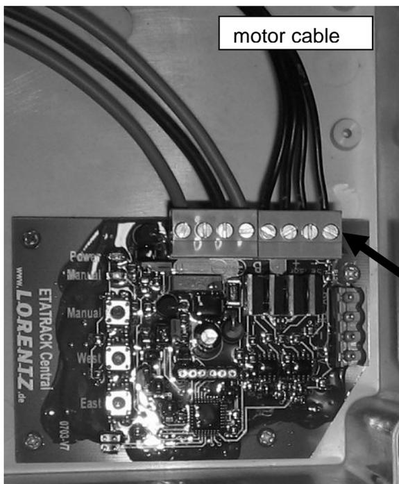
The motor cable must be plug on right upper terminal.
