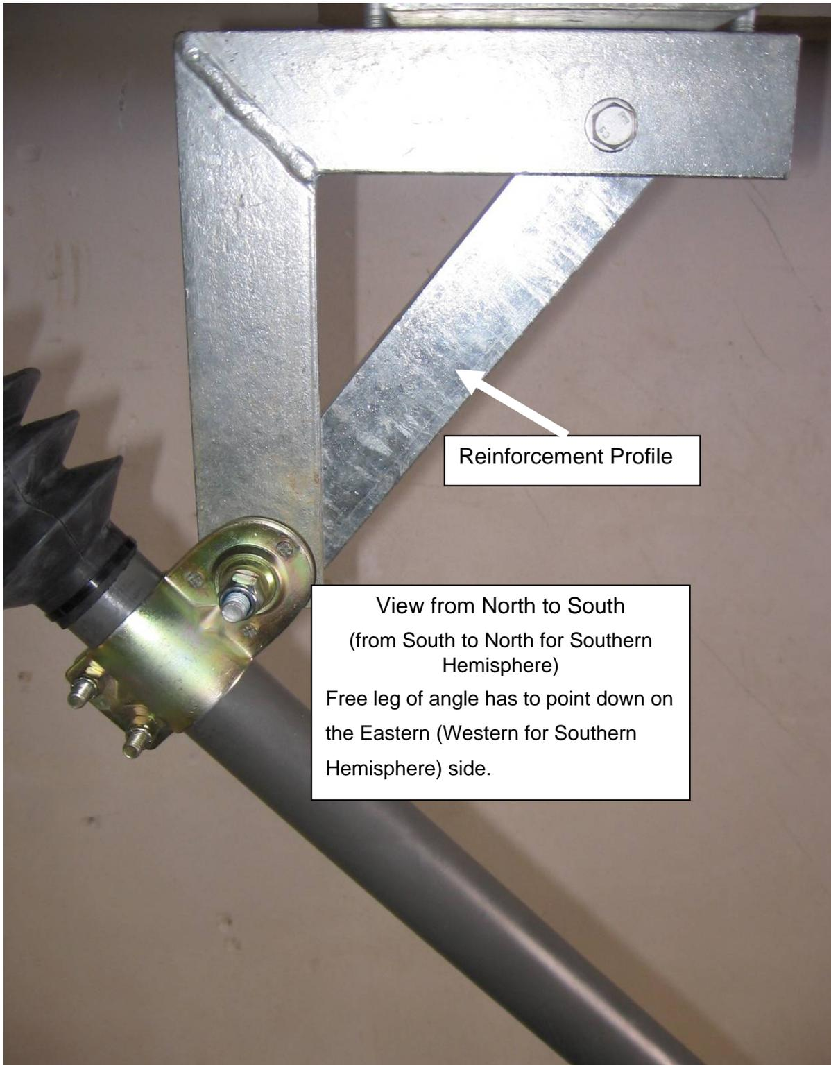
Fig. 5.4 Arrangement of lower motor fixation
